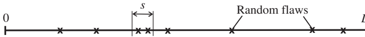
Figure 16.11 Clustering within a critical distance s of two or more random flaws following a homogeneous Poisson process in a piece of thin wire with length L .
