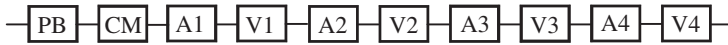
Figure 2.13 Reliability block diagram related to the delivery of working fluid through both pipelines.
